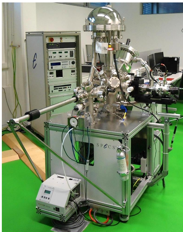
Figure 3.5 Used Specs X-ray Photoelectron Spectroscopy (XPS) equipped with a hemispherical energy analyser PHOIBOS 100 MCD-5 [159].
