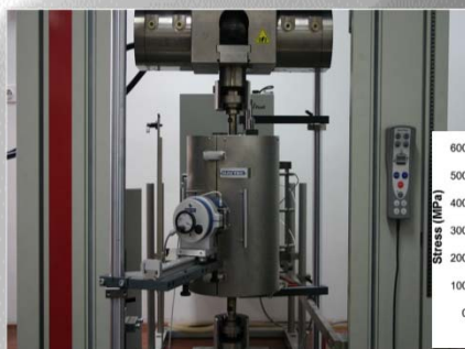
Testing system for characterization of mechanical behaviour at elevated temperatures
