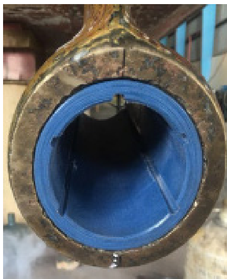
Fig. 11. Bearing made of composite material lubricated with seawater (source: [12])
