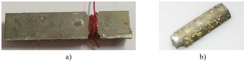
Figure 4. NiTi rods: (a) After 6 months of exposure, (b) After 12 months of exposure
